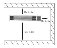
For safe use of the product, the product installation position should have a minimum height of 1.8 m from the ground, and a minimum distance of 0.5 m from both side walls, ceiling and roof.
